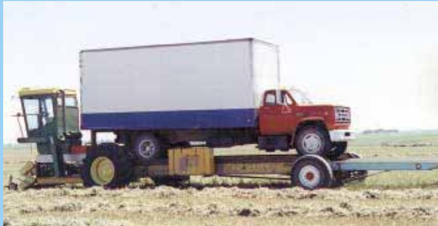
Alexander carries a 3-ton truck on back of his modified Deere 5400 self-propelled forage harvester. When the truck gets full, he drives it off the 22-ft. long deck and heads back to the farm.
