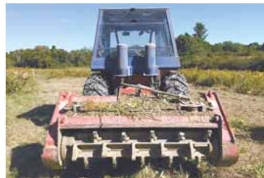
System includes loader-mounted tanks, as well as a shredder/mulcher equipped with brush guards. It's used to plane down exposed and protruding roots.
