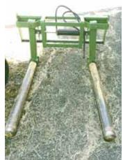
Equipped with rolling pipes instead of grabbers, Allen Pansegrau's big round bale lifter avoids messing up the plastic on silage bales.
