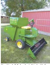
Combine's 5-ft. header is fitted with three 21-in. reel mowers mounted side-by-side.
