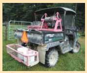
Wilson also built a rear rack for his wife using angle iron on a base frame of 2 by 2-in. tubing that fits the UTV receiver hitch. It holds 5-gal. pails for hauling supplements.
