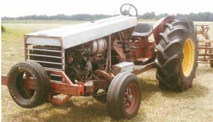
Raymond Bishop built this tractor by attaching the rear end and transmission from an IH 340 tractor to the front suspension system off an old Chevy Impala. Power is provided by a 4-cyl. Pinto engine.
