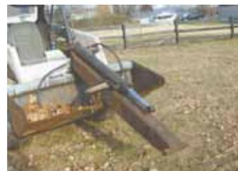
Jackson Brown made brackets to mount an old worn-out backhoe to his skid loader bucket (left). Bucket can be quickly removed.
