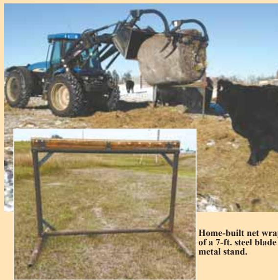
Inventor Dick Schirado uses a grapple fork to pick up bales and slides it over top of blade to cut through net wrap.
