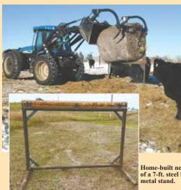
Inventor Dick Schirado uses a grapple fork to pick up bales and slides it over top of blade to cut through net wrap.
