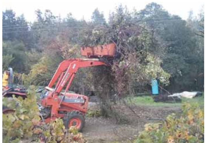
To grab a pile of brush, Bernier backs up with the weights dragging along the ground, until they trap brush inside bucket.
