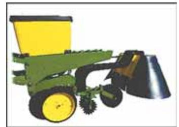
Mounted on planter row units, Cotton Tail hoods confine spray treatments to small, isolated bands that reduce drift during application.
