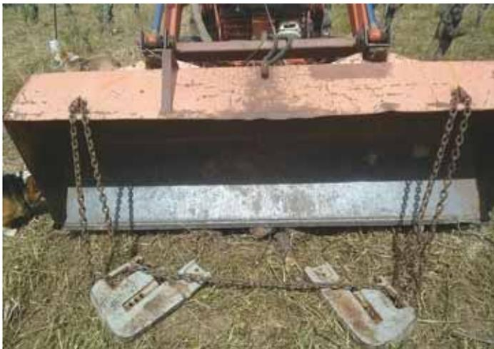
Bernier attaches chain and a pair of 70-lb. tractor suitcase weights, to his loader bucket to hold big loads in place.
