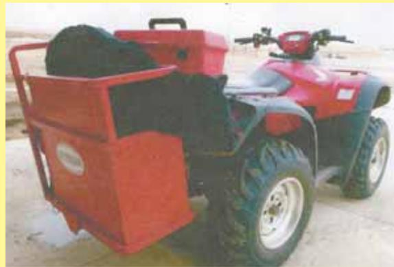
One end of calf hauling crate has a door with an opening on top large enough for a calf to look through. Unit hooks up to the receiver hitch on an ATV or pickup.
