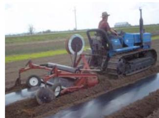
“This 65 hp crawler will outperform any 4-WD tractor in the produce patch. It has less slippage and reduces soil compaction when tilling ground. Our fields are usually a little on the wet side early in the spring and, with the crawler, we can till fields one or two days earlier.
