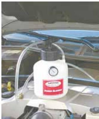
**Power Bleeder consists of a pressurizer jug with a hand pump and pressure gauge, bleeder tubes, and a hose with a cap fitting to match the brake cylinder reservoir neck.**
