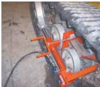
**Hydraulic-powered rubber track installation tool makes it easy to install all kinds of tracks.**
