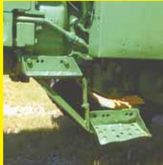
Due to health issues, I needed to reduce the height of the first step on my Deere 3020 tractor. I moved the right hand step, which was never used, to the left side. Using some flat iron, 4 bolts, and welding an angle brace, I was able to reduce that first step by 8 in. The ground to first step is now 17 vs. 25 in. The same idea can be used on a 4020. (Ron Roberts, 1518 S. Prairie Rd., Stillwater, Okla. 74074, ph 580 371-5333).
