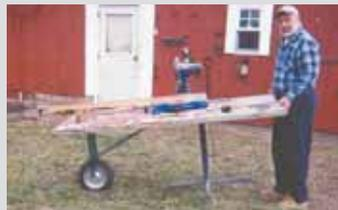
I keep it outside most of the time and use it to work on various projects. The big wheelbarrow wheel makes it easy to move from work area to work area as needed, and if I want I can also use it as a scaffold to paint buildings.
