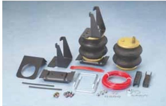
**Ride-Rite airbag kit levels and balances loads to reduce "bottoming out" and increase vehicle stability.**
