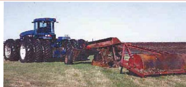
Chuckry's "deep plow" is used at about 5 mph and can plow 25 to 35 acres a day. A 40-ft. steel roller trails behind.
