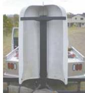
Dale Hiatt made this trailer-mounted bug deflector by bolting together 2 air deflector side panels off a semi truck. Deflectors are supported on back by an angle iron frame.
