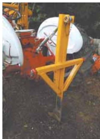
Connor Bishop used 2-in. sq. tubing to build ripper frame and bolted a homemade blade to it. Tractor's 3-pt. lift arms attach to sq. tubing with square "washers."
