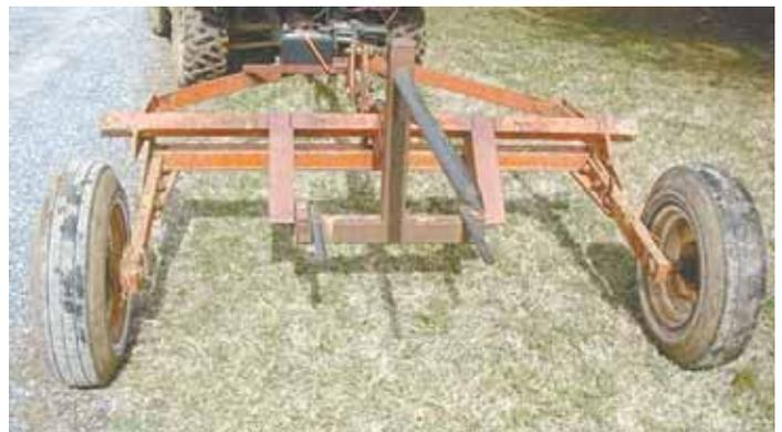
He removed seed boxes from the planter and welded braces to the bottom of the planter carriage, then bolted on a 3-pt. bale spear.
