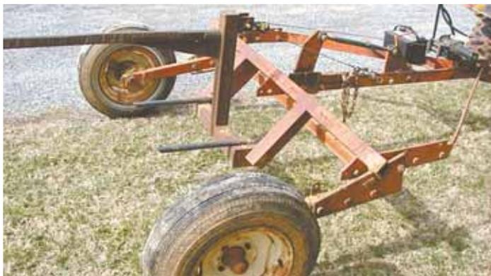
Billy Mayhew converted an Allis Chalmers 4-row corn planter into this 2-wheeled round bale mover. A remote-controlled electric winch is used to raise and lower the bale.
