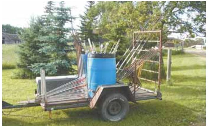
His fencing cart has an assortment of racks, each designed to hold specific posts and gear.
