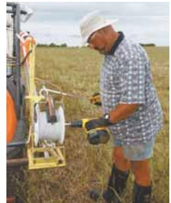
Polybraid wire reel holder mounts on front of an ATV or utility vehicle and is operated by a cordless drill.
