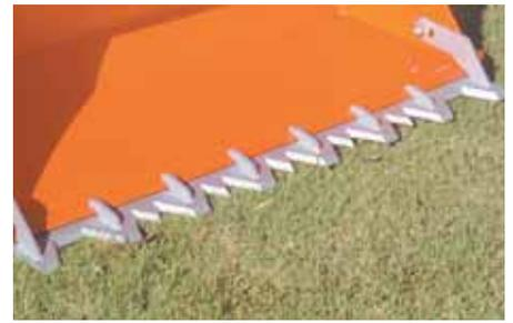
**Loader bucket-mounted Piranha tooth bar works great to clear brush and rake out roots.**
