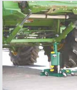
**Emerson's 60,000-lb. twin cylinder air-over-hydraulic lift is designed to handle today's big farm equipment.**
