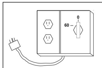
you shouldn't charge the battery for more than 1 hr. or it will be harmful to the battery. I didn't want to have to remember to unplug it so I made a timed receptacle by wiring an electrical box to a timer and then running a plug from the timer to another outlet. I simply plug the battery charger into the timed outlet and set it for an hour."
