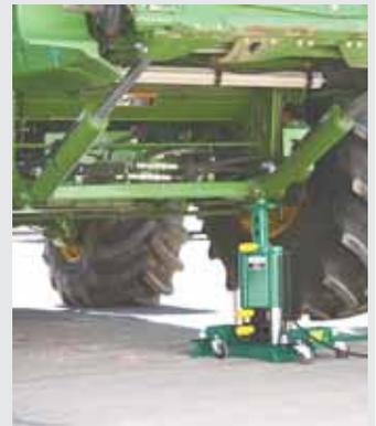
**Emerson's 60,000-lb. twin cylinder air-over-hydraulic lift is designed to handle today's big farm equipment.**
