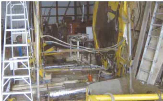
With all the bale-forming belts, belt guides and rollers removed from the bale chamber, Axelson used threaded rod and flat iron to hold the baler's walls in place.
