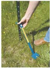
You hold the T-post Badger down with your foot and use a pushing and pulling action against post. As post emerges from ground, the top of the tool ratchets down post's knobs.
