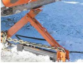
Offset jack works somewhat like an ordinary scissors car jack, but operates off tractor hydraulics.
