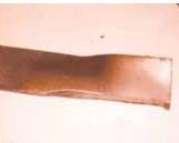
Unsharpened "finger" at end of blade knocks stones out of the way and acts like a hook to pull grass into blade.
