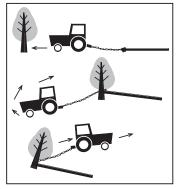
Drag a heavy pole behind a tractor with a log chain and drive around trees and brush to yank them out.
