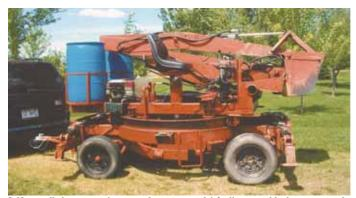
Self-propelled excavator is mounted on a powered 6-ft. dia. turntable that supports the boom. A pair of 55-gal. barrels on back are filled with water to serve as counterweights.
