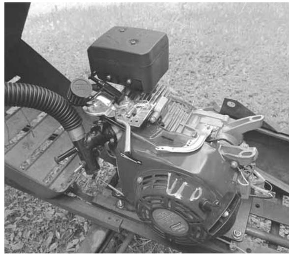
Filtered gas runs through hoses into the tractor's engine, a 6 1/2 hp. Honda clone. Davis fabricated a carburetor to better match the engine to the charcoal gas output.
