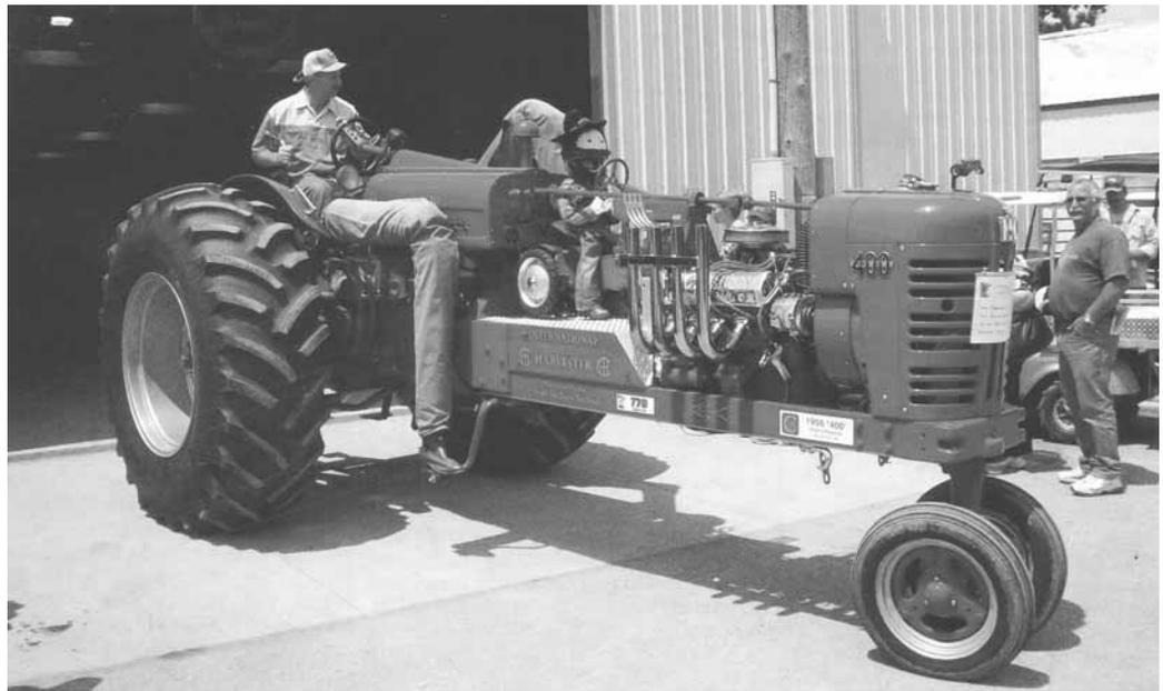
**Stretched-out Farmall 400 is powered by a V-8 engine and an automatic car transmission, with a Farmall pedal tractor above it. A pair of custom "legs" operated by a 12-volt motor move 2 large pedals underneath the tractor.**
