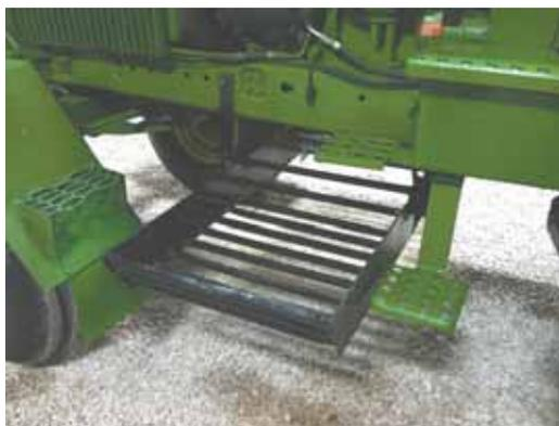
Heavy-duty rock carrier mounts under Deere 4440’s frame behind the front wheels. Pipes are spaced 2 in. apart to allow any dirt to drop out onto the ground.
