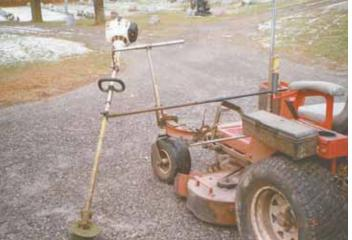
Trimmer hangs from a T-bar mounted just ahead of mower's front wheel.
