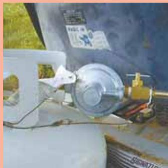
A small propane tank mounts on back of Bodell's lawn tractor, along with a regulator and hose that leads to the tractor's air cleaner.
