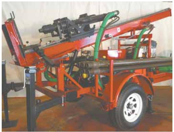
Compact Aqua Bore well drilling rig is small enough to be carried in a pickup bed or towed on a trailer by a pickup or small tractor.
