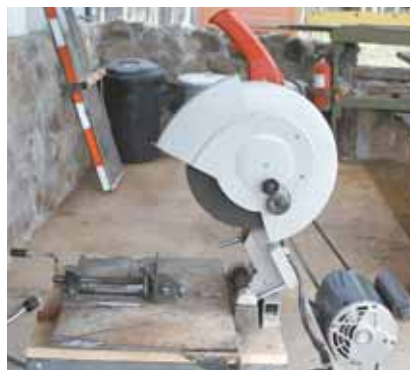
Salvaged parts from a pair of Milwaukee chop saws were used, including the handle, blade guard, switch, and tilt pivot pin and spring. The rest was made from scrap steel remnants.
