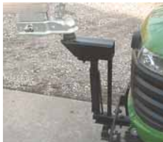
Tongue swivels on a 2-in. ball mounted on front of mower. Push mower end of tongue bolts onto a piece of plywood that's free to swivel up or down via a pair of barn hinges.
