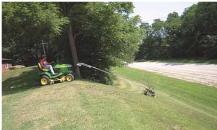
James Lake uses his Deere riding mower, fitted with a push mower at the end of a 16-ft. long tongue, to mow a steep hill in his front yard.
