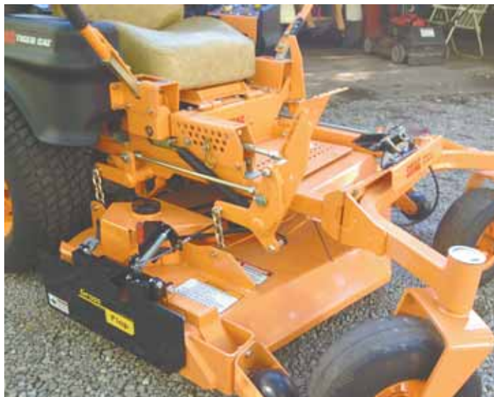
Foot pedal lets you open and close the flap on mower's grass discharge chute with your feet while steering in close quarters.
