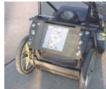
Tongue swivels on a 2-in. ball mounted on front of mower. Push mower end of tongue bolts onto a piece of plywood that's free to swivel up or down via a pair of barn hinges.
