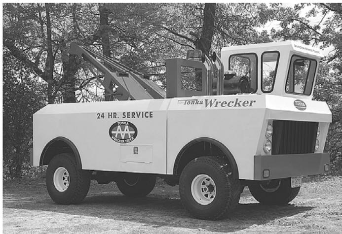
Brad Doane built this 16-ft. long, 10-ft. tall and 2-ton life-size replica of an old Tonka Wrecker tow truck. It's set up with a hand-cranked winch.
