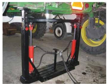
Sprayer lift is designed to operate off tractor hydraulics and is equipped with slots that also fit a forklift or front-end loader.
