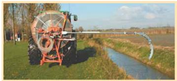
Power Jetter works like a giant snake to unplug drainage tile without digging it up. It slowly pushes a solid plastic hose into tile line while injecting a stream of water at up to 500 psi.
