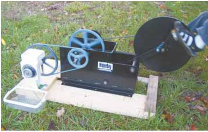
Pedal-powered pto work station can be used to operate any low rpm tool, including alternators, grain grinders and even power shop tools.
