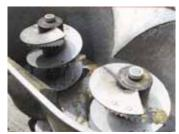
Mixer uses 2 stainless steel augers with serrated cutting knives to cut up baleage and dry hav.
