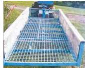
Flooring varies from plywood to used rock crusher screens. "The trailers work great for hauling lumber slabs and firewood, savs Stubbs
