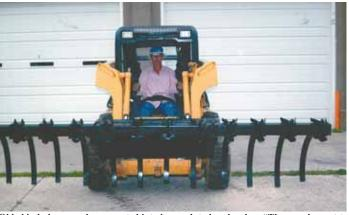
Old chisel plows can be converted into heavy-duty brush rakes. "They work great to
