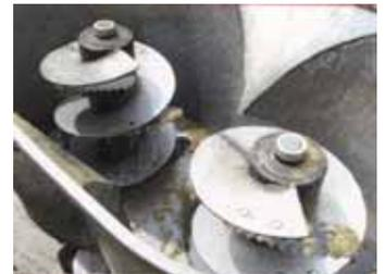
Mixer uses 2 stainless steel augers with serrated cutting knives to cut up baleage and dry hay.
