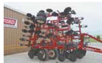
Opposing coulters build the berm, and mole knife shanks break up wheel track compaction. Salford now offers a tillage tool based on Muench's design (right).
