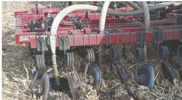
Strip-tilling in continuous corn residue is difficult, but Mark Muench solved the problem by mounting opposing coulters on a Salford strip-till tool.
