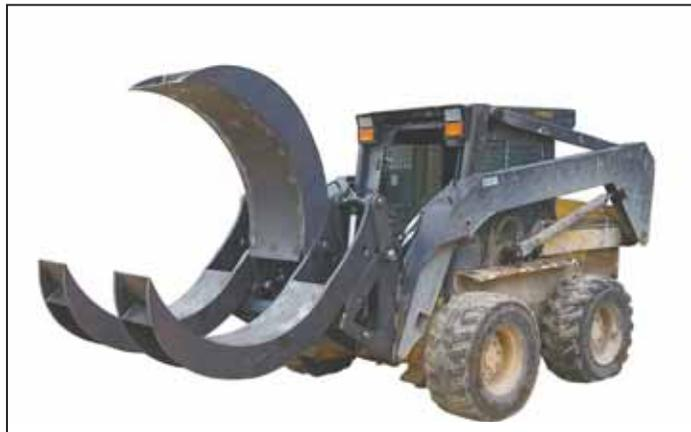
Smidley Piece Maker has an upper jaw that closes between two lower jaws to break up carcasses.
