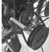
Glenn Sherwood built this motorized bicycle that's powered by an old 8 hp Tecumseh engine. It belt and chain-drives the bike's rear wheel.
