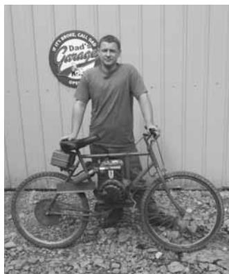
Glenn Sherwood built this motorized bicycle that's powered by an old 8 hp Tecumseh engine. It belt and chain-drives the bike's rear wheel.
