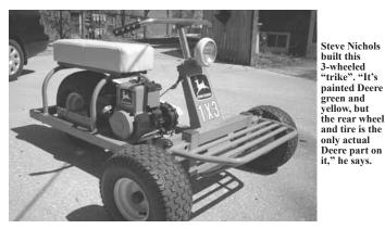
rear axle and bearings, the 12-in. pulley and V-belt, and the conduit elbows which form the seat support. Everything else was salvaged mower parts or things I fabricated from odds and ends. The headlamp is just for
