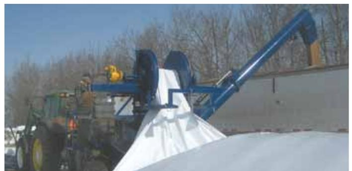
Neeralta Mfg.'s new grain extractor can unload a 9 to 12-ft. dia. grain bag at up to 150 bu. per min., then roll the empty plastic bag up into a neat 30-in. wide roll.
