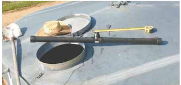
Floats are made out of pvc pipe and partially filled with water and bleach to make them heavier.
