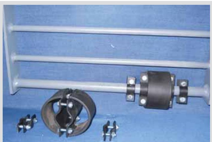
Add-on “split wheel” is designed to fit onto the bottom round crossbar on swinging gates. The 2 parts bolt together and are held in place by 2 clamps.
