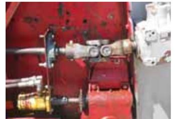
Because of the angle of the framework, they had to put a double yoke on the beater driveshaft before it enters the gearbox.
