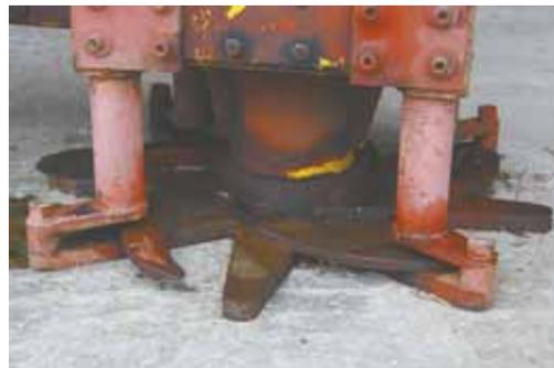
Mounted on a backhoe, the No-Throw brush cutter cuts brush or chips it in place. Unit's 6 curved knives grab and hold branches and trunks as they're cut.
