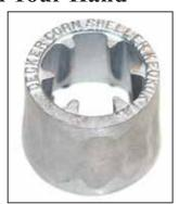
To use the mini sheller, you twist the ear through the collar and let sheller's 6 ridges rub the kernels off.
