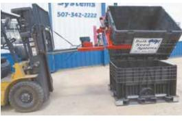
Seed box flipper slides onto standard forklift forks. Arms powered by an electric actuator open and close to grip seed box.
