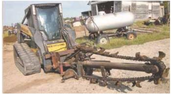
"It does the work of much more expensive machines," says Chuck Hardenburger, who converted an old 3-pt. trencher into a skid loader-mounted model.
