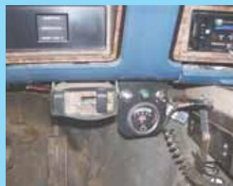
A master toggle switch was installed on the dash. Unless it's turned on, no LP gas can flow. A brake light switch installed on the accelerator pedal linkage controls the solenoid valve (right).
