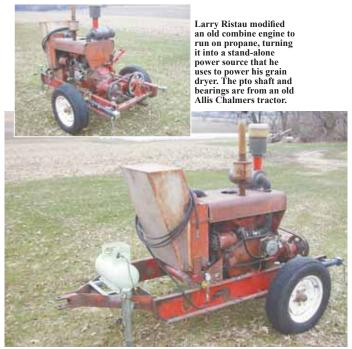
valve to the mini-tank and vapor feeds into the carburetor to start the engine.
