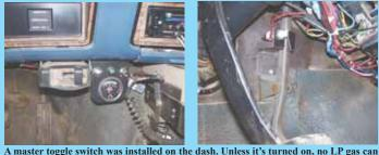
A master toggle switch was installed on the dash. Unless it's turned on, no LP gas can flow. A brake light switch installed on the accelerator pedal linkage controls the solenoid valve (right).
