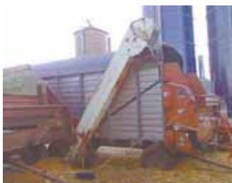
**Low-cost seed handling system uses the elevator off an old corn picker alongside a covered chopper box. Picker's husking beds, as well as a sorting table and an unloading conveyor belt, are suspended off the floor inside the chopper box.**
