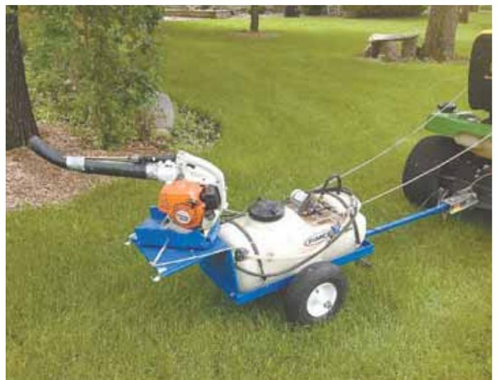
Leaf blower mounts on a turntable at back of sprayer and, by pulling on a pair of ropes from the tractor, can be rotated back and forth up to 180 degrees.
